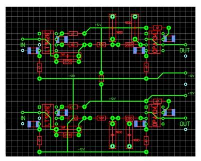
The decoupling to ground of the power connections of the op amp's has been made with 1 uF SMD chip-C's.
