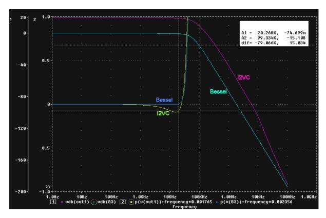
The blueish curves belong to the theoretical third order Bessel function for fl = 60 kHz. Such a function is phase linear until fl/3 = 20 kHz as is shown by the blue curve. The light-blue curve shows its amplitude.
