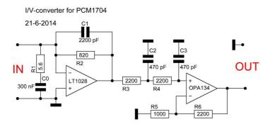
The current of a PCM1704 is only ±1.2 mA so that the gain will be less than with a PCM1792. One could change R2 for more output from the I2V but mind the phase linearity! (See "I2V-details on subelements" on this site.) It is more simple to change the gain of the OPA134 adding R5 and R6. The (high) output of 8.8 V<sub>ff</sub> at 0 dB, as with the PCM1792, will be obtained again.
