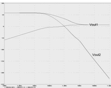
The input resistor (here R12) would start the roll off a bit to early (2 dB loss at 20 kHz) so that the feed back resistor (R11) has been changed to 820  $\Omega$  which yields: 88 kHz together with 2200 pF. This low value has also been chosen because of the larger current of DAC's like PCM1792.
